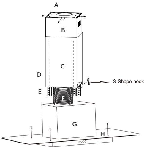
4. If the glass canopy has not been pre-assembled by the factory, then it should be attached to the top of the main body of the range hood at this stage.
