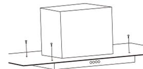
5. Lift the main body (G/H) of the range hood onto the support frames (D/E) and fix into position using [16] M5 screws.
