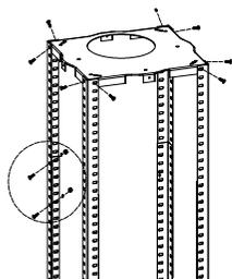
**IMPORTANT: The angle bars must have an overlap of AT LEAST 100mm/4"**
