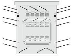
**3.** Install a UL listed strain relief (not provided) to the power cord opening in the bottom panel, and then completely tighten the nut.
