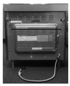
The range is supplied with an antitilting chain to prevent the appliance from tilting forward and accidental damage to the gas pipe. Take the wall anchor with hook and make an adequate hole in the wall behind, at the same height as the chain. Insert the wall anchor into the hole and screw in the hook until it is firmly fixed to the wall. Connect the chain to the hook.
