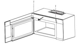
4 Remove the charcoal filter by pushing it inwards, then lift up and pull it out of the microwave.
