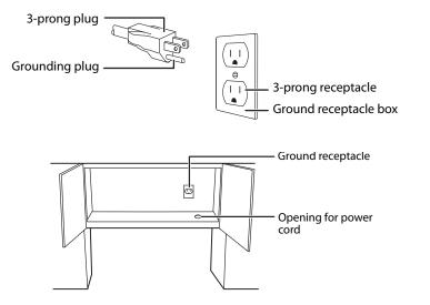
If the power supply cord is too short, have a qualified electrician or serviceman install an outlet near the appliance.
