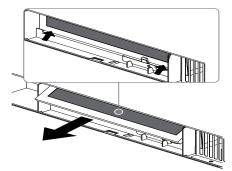
5 Push the tab to release the light cover and carefully pull it up from the front edge.
