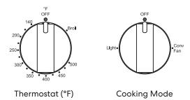
Turn the oven Thermostat knob and Cooking-Mode knobs to set the temperature and oven mode. The oven will turn on, and will automatically shut off according to the time set. When the shut off time is reached, press any button to stop the beeping and return the oven knobs to the OFF position.
