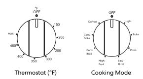
Turn the oven Thermostat knob and Cooking-Mode knobs to set the temperature and oven mode. The oven will turn on, and will automatically shut off according to the time set. When the shut off time is reached, press any button to stop the beeping and return the oven knobs to the OFF position.
