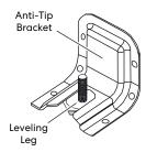
Making sure the anti-tip bracket is installed:
