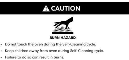
The Self Clean cycle uses very high temperatures to burn soil to a powdery ash and clean the oven's interior automatically.
